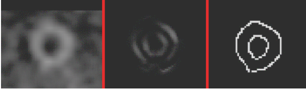
Figure 6: Original SPECT image (left), after Reynolds operator (middle) and after Canny operator (right).
