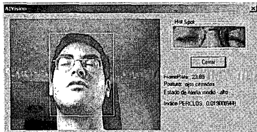
Fig. 5. The application shows the personal profile, the eyes pose, the PERCLOS index, the warning level assigned and the frame rate.
