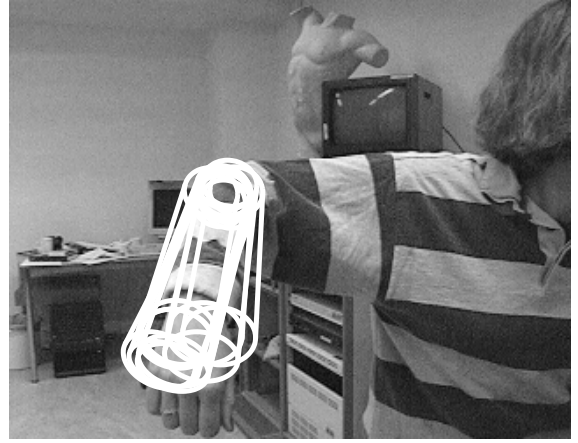
Figure 5. Illustration of a sampled distribution: 10 samples from a posterior distribution over \boldsymbol{\phi}_t for an arm, projected into the image coordinate system.
