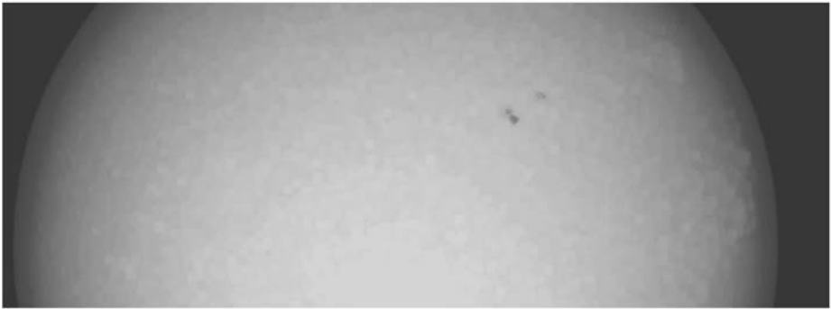
Figure 3 Dilated image using a square SE sized 11 \times 11 once this operator is applied over the fragment of the original image obtained at Ebro Observatory on 19 October 2001.
